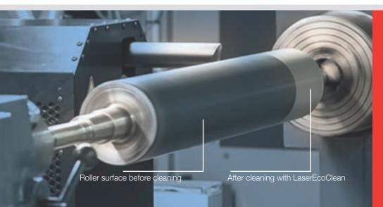
The cells on the anilox roller can become clogged with ink residues during use, which reduces the volume of the cells concerned. After laser cleaning with LaserEcoClean technology you take full advantage of the pick-up volume of your anilox rollers, and thus reap the same benefits as you would at the beginning of uniform colouring in the printing process.
